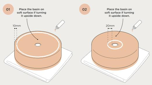
Run a line of clear wet area silicon around the underside of the basin 10mm back from the edge.
