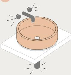
Install waste in a compliant manner. Waste must be hand tight only and not overtightened with tools.
