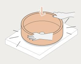
Press basin down into benchtop and remove excess silicon using wax and grease remover and soft cloth.
