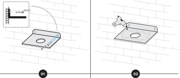
Bolt bracket to tiled wall, ensuring bracket is placed at level height. Be sure to tape over tiles before drilling.
