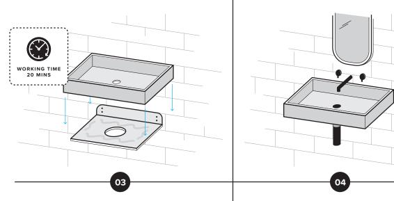
Lower basin onto glued brackets, ensure placed centrally. Working time: 20 mins
